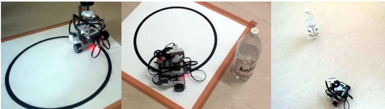
Figure 3: Computing circle diameter: using Tales circle (left), using circumference (middle), measuring width as the altitude in a general triangle with all sides known (right). NXT-based robots were used here.
