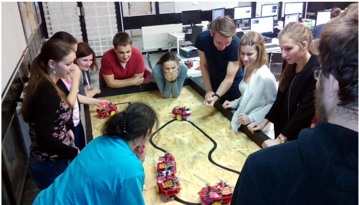
Figure 1: Student exercise, participants programmed their robots to follow line and navigate a maze.
