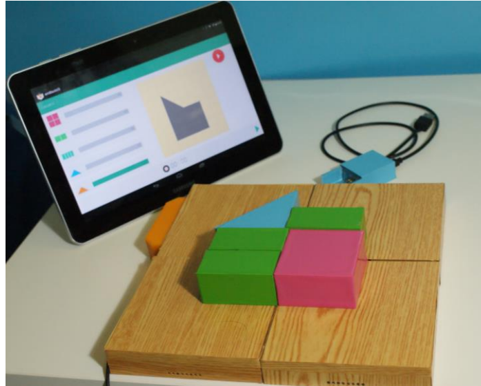
Figure 1. eM tool Designed as a Tangible Environment for Learning Linear Algebra, where blocks in each color have distinct numerical values, and their juxtaposition corresponds to the sum of those numbers. This tool comprises 3 parts: blocks, base, and the mobile application.
